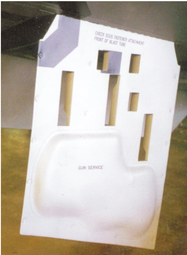
Gun breech cover panels, full size on the left
